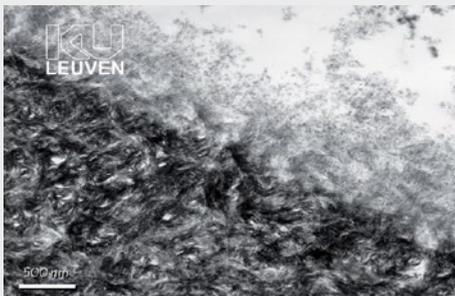
The transmission electron microscope (TEM) shows the interface image of CLEARFIL™ SE BOND.
