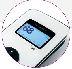
**3.** An ISQ value is generated and shown on the display. It reflects the level of stability on the universal ISQ scale – from 1 to 100. The higher the ISQ value, the more stable the implant.
