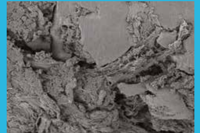
Implant retrieved after 8 weeks shows new bone ingrowth inside the surface cavities.
