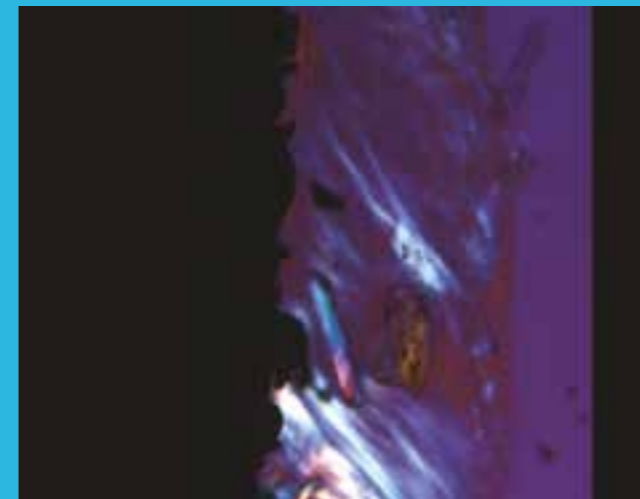
The connective fibers get perpendicularly on the TiXos surface.
