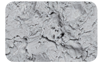
Anthogyr BCP ® implants surface microscopic observation
