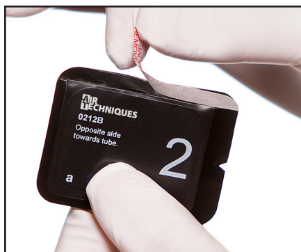
Figure 7b Peel off the adhesive strip.
