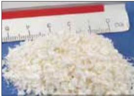
After particing, volume gain was about 7 times.
