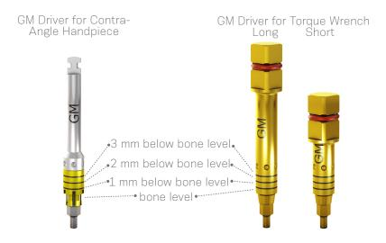
Note 1: There are 3 similar markings at 1-mm intervals in the Drivers for the Contra-angle handpiece and Torque Wrench. These markings guide the depth of the final positioning of the implant in the following way: first stripe for 1 mm below bone level, second for 2 mm and third for 3 mm. Each full turn of the implant results in: (a) 2.2 mm for the Drive implants; (b) 1.4 mm for the Helix implants; and (c) 1.2 mm for the Titamax implants.
