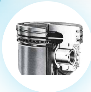
Sealing effect of a piston ring
