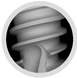
SEM magnificationX25: clean uniform surface with no contaminations
