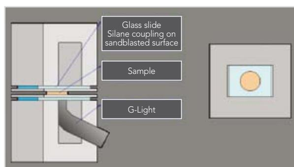
Figure 2. Three-body wear resistance test set-up.
