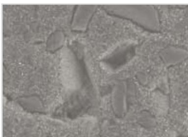
5b. Clearfil Majesty Esthetic† x1000 after 100,000 cycles. Note the loss of pre-polymerized fillers and gaps at the interface of the particles and the resin matrix.
