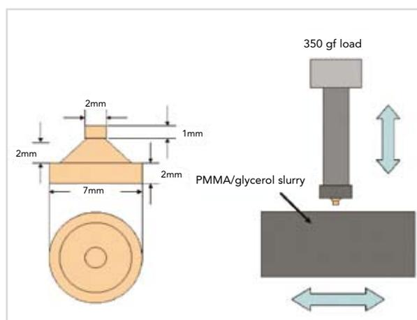
3. Combined polish retention/surface roughness test
