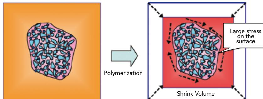
Figure 9b. Polymerization shrinkage stress with KALORE.
