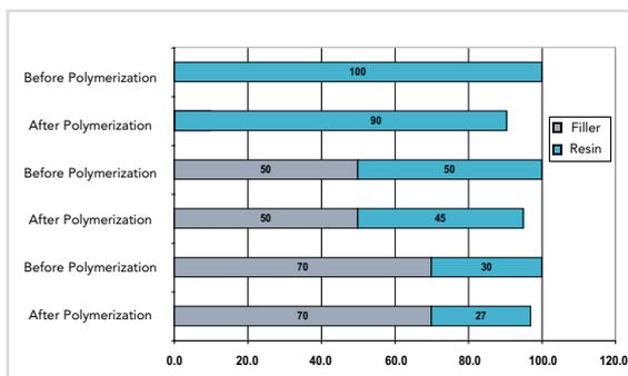
Figure 5. Polymerization shrinkage of low vs. high molecular weight monomers.
