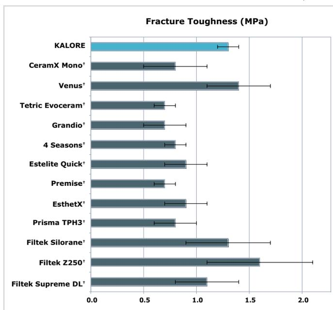
Figure 18. Fracture toughness.
