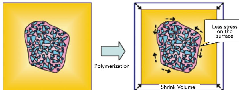
It can be concluded that DX-511, the new low shrinkage monomer, is effective in reducing shrinkage stress as demonstrated by testing of KALORE. The reduction in ongoing stress within the composite resin helps retain fillers in the matrix, especially after stress is applied to the cured composite resin. The surface smoothness, wear resistance and polish retention were also found to be superior with the addition of DX-511 to the composite resin formulation.
