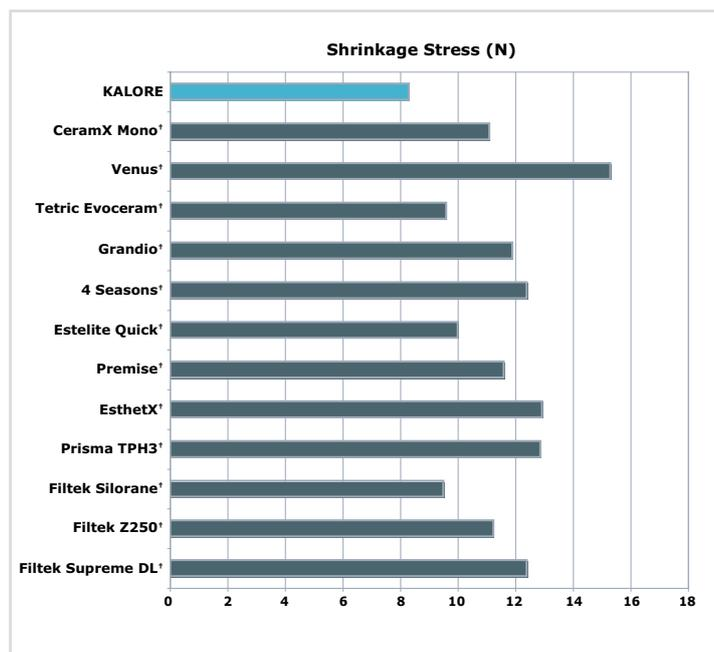
The sample was light-cured for 40 seconds from the underside using a G-Light™ 11 mm fiber rod, then light-cured for 20 seconds from above. The setting shrinkage stress was measured for 20 minutes and the highest figure reached was recorded as the shrinkage stress. **KALORE demonstrated the lowest shrinkage stress of all products tested (Fig. 14).**
